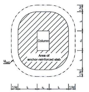
Critical perimeter u<sub>1</sub> and outermost perimeter u<sub>out</sub>
