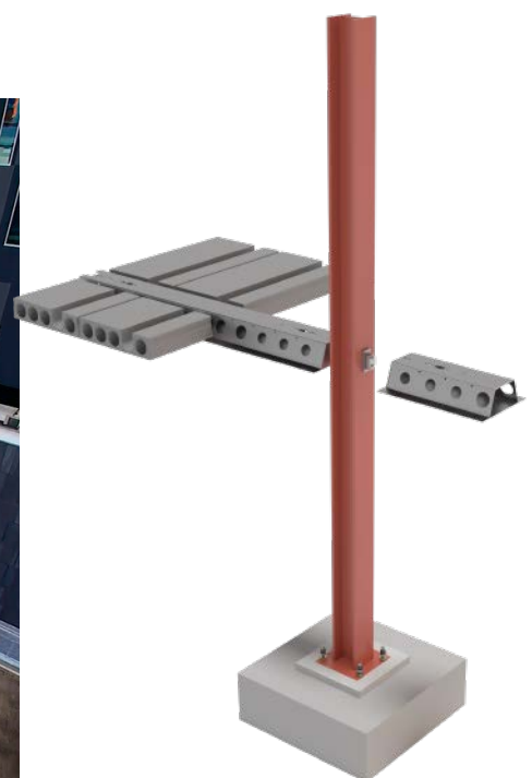
FIGURE 17 SIDE VIEW TO CONSTRUCTION SITE OF GLASSHOUSE (LEFT). DELTABEAM®— STEEL COLUMN CONNECTION (RIGHT).
